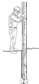
NOTE: If desired, a second pole key anchor may be used at the top (ground level) of the hole on the opposite side
