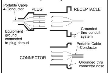
**Style 1 Plug** - Equipment grounding conductor is wired directly to the ground terminal which is connected to the ground stand-off and shroud. This, in turn, grounds the entire plug assembly housing. All contacts are "current carrying".
