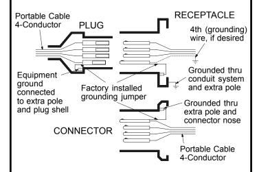
**Style 2 Plug** - Equipment grounding conductor is wired to the extra grounding pole terminal which provides a parallel ground circuit thru the extra ground pole and plug shroud. The ground stand-off and shroud are grounded to a copper alloy ground jumper installed on the extra ground pole. This, in turn, grounds the entire plug assembly housing.
