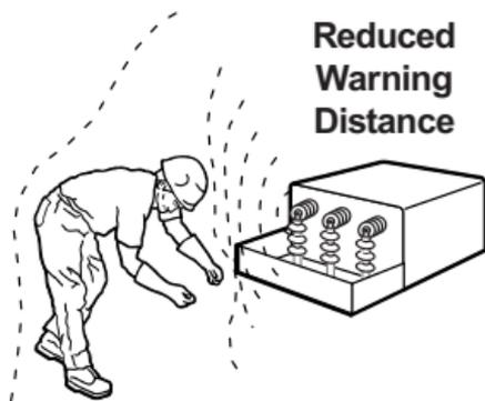
The V-Watch Personal Voltage Detector measures only the strength of the electric field. It cannot directly measure distance to the source of the electric field such as an energized conductor. The higher the voltage, the stronger the field and the greater the alarm
