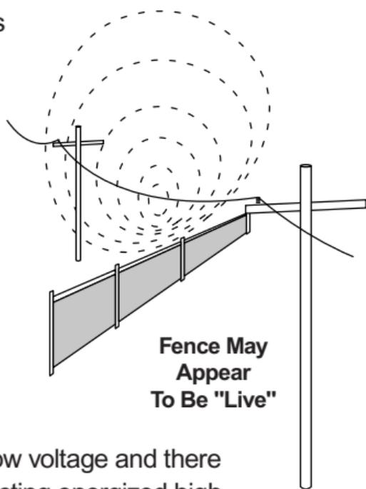
As an additional protection against false alarms from transient voltages, the detector has a built-in time delay and may take up to one second to emit an alarm warning of high voltage. For this reason, a user running towards an energized high voltage source may find the warning distance reduced.
