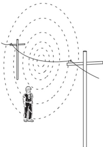
A downed power line is a typical hazardous situation where the detector can provide a warning. This power line lying on the ground sets up a high voltage field surrounding the conductor that the detector will sense and warn the user.
