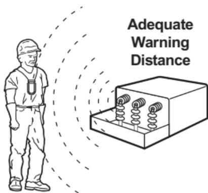
If the user bends over from the waist to reach towards an energized high voltage terminal, the warning distance may also be significantly reduced. In both cases, the high conductivity of the body acts as a shield to conduct the electric field around the detector.
