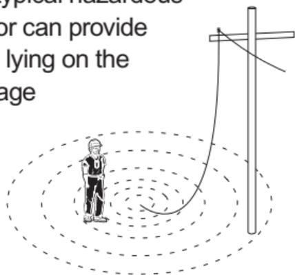
The detector is designed to be worn on the body and it measures the electrical fields typically found in close proximity to the body. Because the human body is a good electrical conductor, electric fields are distorted or even blocked by the body. Thus, positioning of the detector on the body and its location relative to the voltage source can have a large effect on its sensitivity to electric fields.
