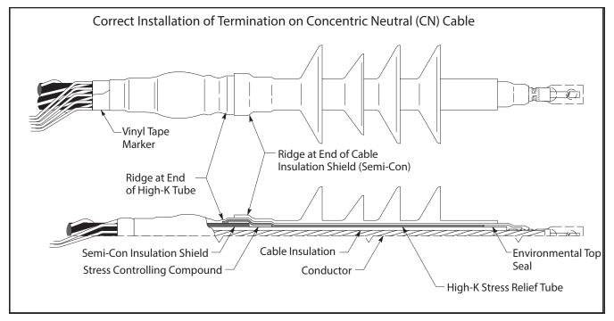
NOTE: Conventional upright operation. The skirted insulator assembly may be installed in the conventional upright position. See pages 12 and 13 for installation instructions.
