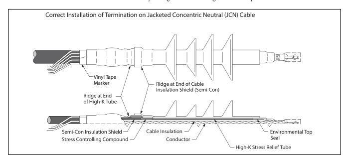
NOTE: Conventional upright operation. The skirted insulator assembly may be installed in the conventional upright position. See pages 12 and 13 for installation instructions.
