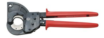
These Klein Tools ACSR Racheting Cable Cutters are equipped to cut up to 477 MCM ACSR multi-strand. They have high-leverage ratcheting mechanisms for easier cutting, and can be locked when not in use. They are size efficient as well, with a length just under 14-Inches they can be carried around in a tool pouch.
