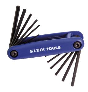
The Klein 70573 Hex Key Set ends are square-cut for a secure, full-depth fit and maximum contact with the hex socket which works to prevent slippage and stripping of the socket while in use. Sizes are: 5/64-Inch, 3/32-Inch, 7/64-Inch, 1/8-Inch, 9/64-Inch, 5/32-Inch. Handy sets fit your pocket or tool box easily and help eliminate the lost-key problem.
