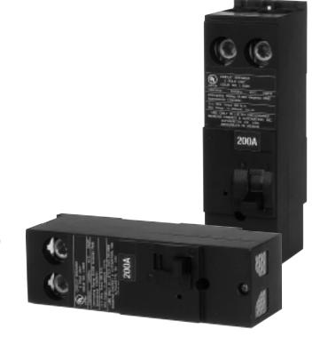
The new circuit breaker family QN2150R thru QN2200R offers the latest in thermal-magnetic circuit breaker design. It directly replaces the now obsolete fully magnetic sensing QPM2150RV thru QPM2200RV and QPJ2150 thru QPJ2200 circuit breaker families. In this new design the handle returns to the center (trip) position similar to our other thermal trip
