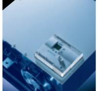
Packed with the highest degree of functionality, the SIRIUS 3RW44 also handles difficult starting operations simply but softly. Thanks to its innovative closed-loop torque control, it can be used to start drives up to a power rating of 900 HP at 460 V in a standard circuit configuration or up to 1600 HP at 460 V in an insidedelta circuit configuration. The functionality designed for simple handling promises to offer the non plus ultra when it comes to operator-friendliness.
