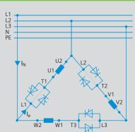
Rated current  $I_e$  of the starter corresponds to 58 % of the rated motor current  $I_N$
