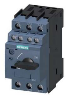
CIRCUIT-BREAKER SZ S00, FOR MOTOR PROTECTION, CLASS 10, A-REL. 1.8...2.5A, N-RELEASE 33A SCREW CONNECTION, STANDARD SW. CAPACITY, W. TRANSVERSE AUX. SWITCH 1NO+1NC
