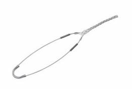
Bus drop, Closed mesh, Single eye. Cable diameter - 9", Mesh length - 3.5", Break strength - 1,100 lbs.
