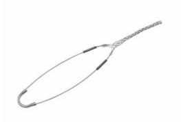
Bus drop, Closed mesh , Single eye. Cable diameter - 0.220-0.320", Bale length - 9", Mesh length - 3.5", Break strength - 1,100 lbs.
