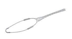
Standard-duty, Closed mesh, Single eye grips. Cable diameter - 1.250-1.490", Bale length - 10", Mesh length - 16", Break Strength - 1,680 lbs.
