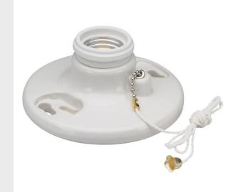
Medium base, porcelain, pullchain, 2 terminals with tri-drive screws, fits 3 1/4 and 4" boxes, with cage neck. White.
