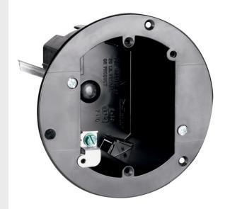
3 3/4" Round Old Work Ceiling box with Swing brackets for mounting that adjust from 1 1/4" down to 1/8". Four Auto/Clamps and Grounding Lug. Includes device mounting holes. 50 pack.
