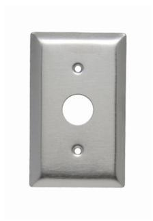
Single gang, single telephone or cable outlet removable 5/8" ID grommet in 7/8" hole. Strap mounted. One #340 yoke. Smooth 302 Stainless Steel.
