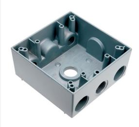
Weatherproof 2 Gang Box, 4 hole 1/2", 30.5 Cu.In., Gray (2 Holes One End, 1 Hole Other End, 1 Hole in Back)
