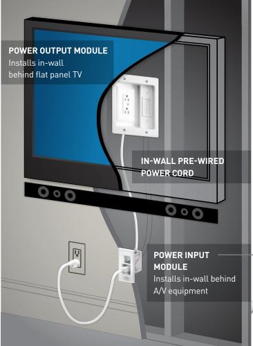
The Power Input Module can also be ganged together for greater flexibility.
