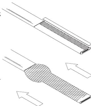
5. At the bulge, separate the braid to make an opening.
