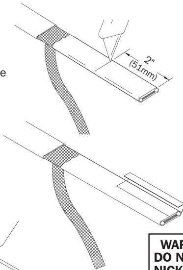
4. Shave the core material from the outside of each bus wire.
