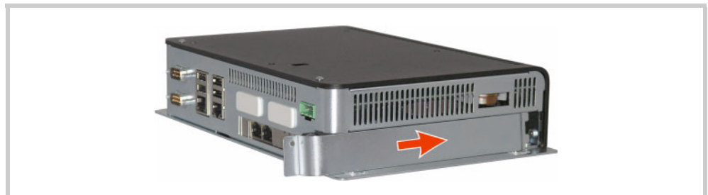
Fig. 24 Positioning the side cover
