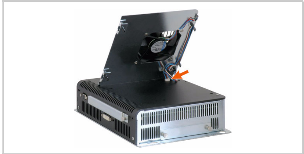
Fig. 30 Power supply for the active cooling unit connected
