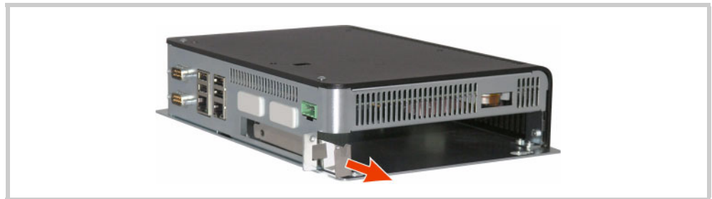
Fig. 22 Removing the PCI card slot cover
