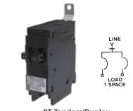
**BT Tandem/Duplex** These space saver duplex breakers combine two independent 1/2" breaker poles in a common unit. This unit bolts onto one panelboard stab and requires one panel space. HACR rated.
