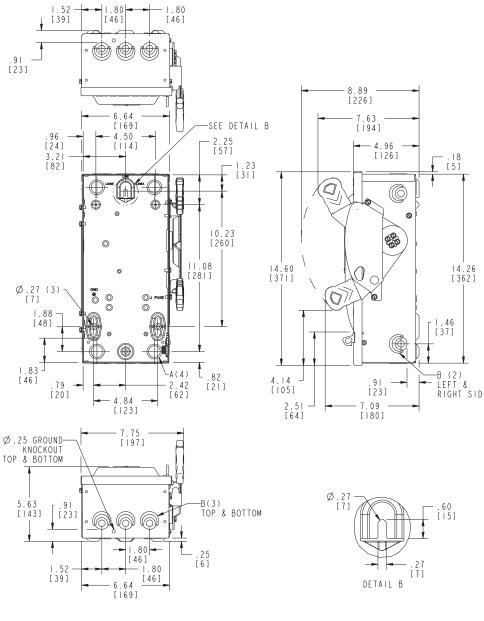
No knockouts in enclosures. Dimensions shown in inches and millimeters ( ). Dimension shown accurate to  $\pm \frac{1}{8}$  in
