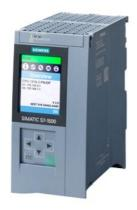
SIMATIC S7-1500, CPU 1516-3 PN/DP, central processing unit with 1 MB work memory for program and 5 MB for data, 1st interface: PROFINET IRT with 2-port switch, 2nd interface: PROFINET RT, 3rd interface: PROFIBUS, 10 ns bit performance, SIMATIC Memory Card required
