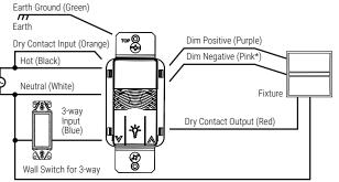
Only one sensor can be used in a 3-way circuit with a switch. The switch will turn on/off the load only at the brightness level selected at the dimmer.
