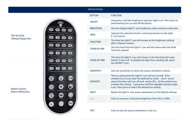
To switch from motion sensor mode to just dimmer mode, long press the ON/OFF button until only the BRIGHTNESS option lights up. If all options light up, long press again. Then use the -/+ buttons to adjust the brightness.
