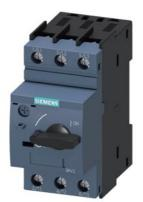
Circuit breaker size S0 for motor protection, CLASS 10 A-release 20...25 A N-release 325 A screw terminal Switching capacity 30 kA at 600 V according to UL/CSA
