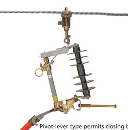
Pivot-lever type permits closing by disconnect stick from side opposite the fusetube. (Plastisol-coated hook lever serves only to close cutout, not to break fuselink.)
