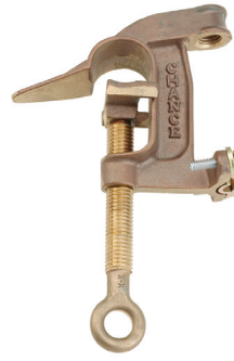
C6002271 Bronze body, Smooth jaws, Bronze eyescrew with fine threads, Tapped for 5/8-11 UNC threaded ferrule
