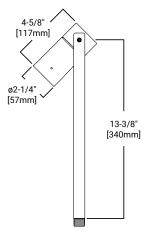
TECHNICAL DATA Low Voltage: 50W Max Halogen MR16 8W LED, L70/60,000 hours at 25°C
