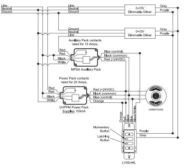
LVSD-ML Wall Station providing vacancy and occupancy control using a UVPPM and MPSA and an OMNIDT series sensor
