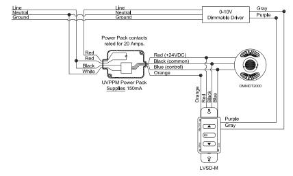
LVSD-M Wall Station providing vacancy control using a UVPPM and an OMNIDT series sensor
