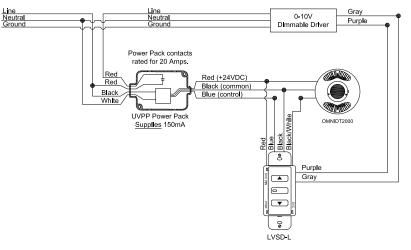
LVSD-L Wall Station providing occupancy control using a UVPP and an OMNIDT series sensor
