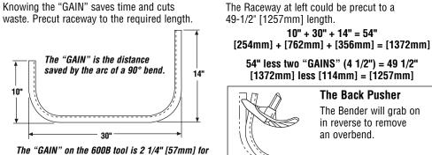
54" less two "GAINS" (4 1/2") = 49 1/2" [1372mm] less [114mm] = [1257mm] The Back Pusher The Bender will grab on in reverse to remove
