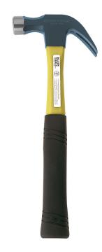
Klein Tools Curved Claw Hammer has adurable plastic-alloy jacketing helps to protect the neck from fraying and splintering if incorrectly struck or overstruck. It has a high-strength fiberglass shaft that absorbs shock and keeps head tight. Hammer comes with a comfortable, perforated neoprene grip.
