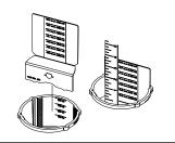
Step 3 Remove the partition and break off the top portion at the first calibration below the mark made from step 2. Reinstall the partition with the small compartment being the communications side.
