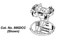
Step 5 Place the gasket support plate over the receptacle and attach with a #6 round head screw.
