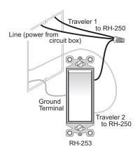
The RH-253 may be used with the RH-250, as shown in these drawings, or with a CH-250, CD-250, CU-250 or RD-250 multi-way sensor in place of the RH-250.
