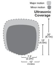
For best performance, Wattstopper recommends using this sensor in spaces no larger than 15' x 15'.
