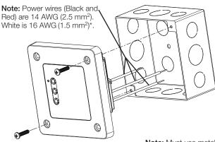
\* Device is grounded via screw terminal
