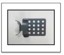
TRM Roof and Gutter Clips are utilized to affix mineral insulated cable and self regulating cable to shingled, seamed metallic, and flat roof tops as well as to the base of gutters if more support is required for the cable.
