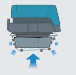
When the power is switched on, Prefilter collapses into itself to compress Damper, and fits closely over Damper and Powder filter.
