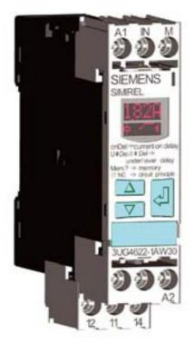
DIGITAL MONITORING RELAY CURRENT MONITORING, 22.5MM FROM 0.05 TO 10A AC/DC OVERSHOOT A. UNDERSHOOT AC/DC 24 TO 240V DC AND AC 50 TO 60 HZ ON AND SPIKE DELAY 0.1 TO 20S HYSTERESIS 0.01 TO 5A 1 CO CONTACT W. OR W/O ERROR MEMORY SCREW CONNECTION REPLACEMENT PRODUCT FOR 3UG3522-1AL20, 3UG3522-1AG20 AND 3UG3522-1AC48-0AA1
