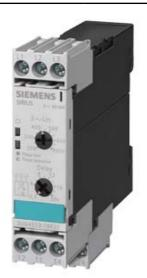
ANALOG MONITORING RELAY PHASE FAILURE AND -SEQUENCE ADJUSTABLE UNDERVOLTAGE UNBALANCE 20% FIXED 3X 160 TO 690V AC 50 TO 60 HZ HYSTERESIS 5% FIXED DELAY TIME 0-20S 2 CHANGEOVER CONTACTS SCREW TERMINAL REPLACEMENT PRODUCT FOR 3UG3013-1B...
