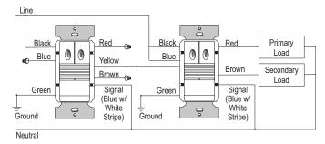
Signal wire connects to neutral. Signal wire can connect to ground in replacement or retrofit application
