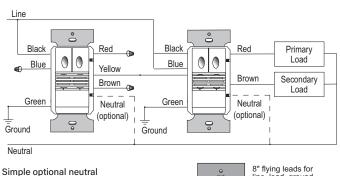
connection allows installation in any 2-wire or 3-wire application.
