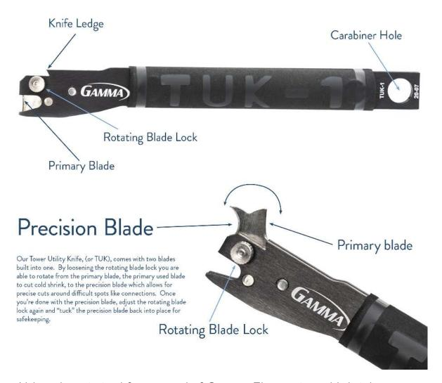
Although optimized for removal of Gamma Electronics cold shrink tubing, the Tower Utility Knife is also very effective at removing Gamma Electronics self-amalgamating Magic Tape®. The Tower Utility knife is not recommended for removal of heat shrink tubing.
