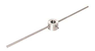
nVent PYROTENAX Pyro Potter (Pot Threading Tool) is a tool used to simplify and improve the installation of brass pots onto copper sheathed mineral insulated (MI) wiring cables. Available in a range of sizes.
