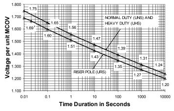
Figure 7. Temporary overvoltage curve. No prior duty –  $60^{\circ}$  C ambient.
