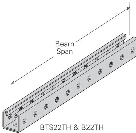
\*Based on simple beam condition using an allowable design stress of 25,000 psi (172 MPa) with adequate lateral bracing (see page 12 for further explanation). To determine concentrated load capacity at mid span, multiply uniform load by 0.5 and corresponding deflection by 0.8.
