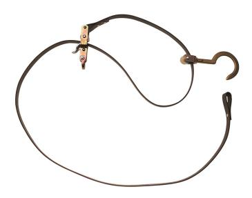
Sag service connections quickly with this simple proven tool. The strap is made of tough nylon webbing, and the swivel hook is forged steel. All metal parts are galvanized, and this tool has a 500-Pound (227 kg) maximum safe load.
