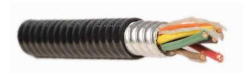
"Metal Clad Cable Type MC is a factory assembly of one or more conductors, each individually insulated and enclosed in a metallic sheath of interlocking tape, or a smooth or corrugated tube."
