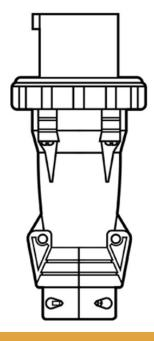
Double pole, Triple wire, Pin and Sleeve Plug. 20 amp, 125 volt.
