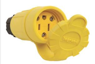
Straight Blade Watertight Connector, 15amp 125volt, 5-15R Configuration, Multipoint sealing system provides environmental protection of: NEMA 4, 4X, 6, 6P & IP67 rated.
