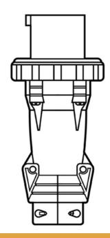
Triple pole, Four wire, Pin and Sleeve Plug. 100 amp, 3Ø/600 vac.
