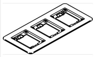
Three-gang brass combination carpet and tile flange, 6.080" x13.310" [154.4mm x 338.1mm]. Accepts Ortronics MAB6TJ TracJack and MAB3S2 Series II, and Wiremold CM Series Open System adapters, sold separately. NOTE: Brass cover plates can only be used with brass flanges. Brushed aluminum flanges come with beveled edges.
